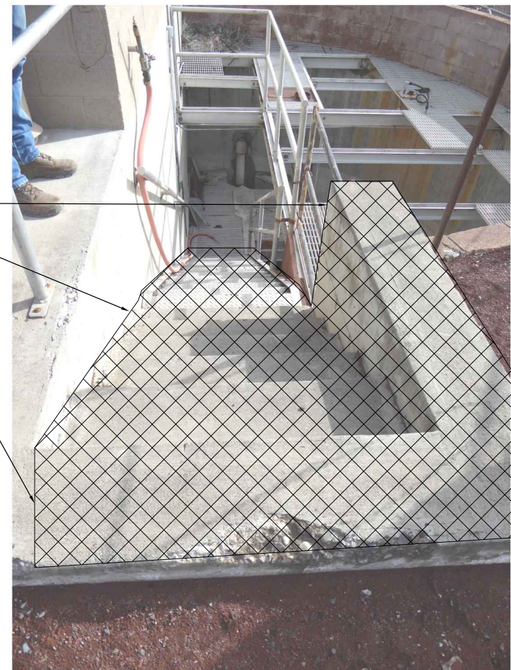
3 DEMOLITION DETAIL NTS
